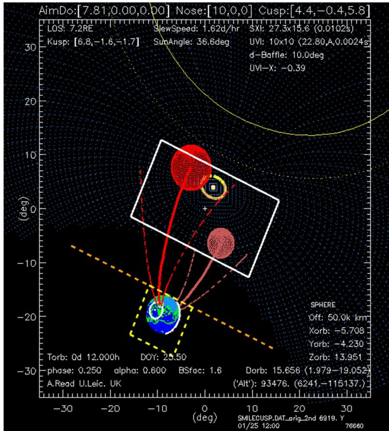
**Fig. 9:** SXI instrument FOV (white rectangle) and UVI instrument FOV (yellow square). The nose of the magnetosphere is shown with a yellow oval at (10.0, 0.0, 0.0)  $R_E$  and the cusps are shown by the red (North hemisphere) and pink (South hemisphere) spheres and by the red and pink magnetic field lines. The SXI Earth avoidance baffle angle is shown with the orange dashed line. The sun avoidance angle is shown by the large yellow unbroken curve.
