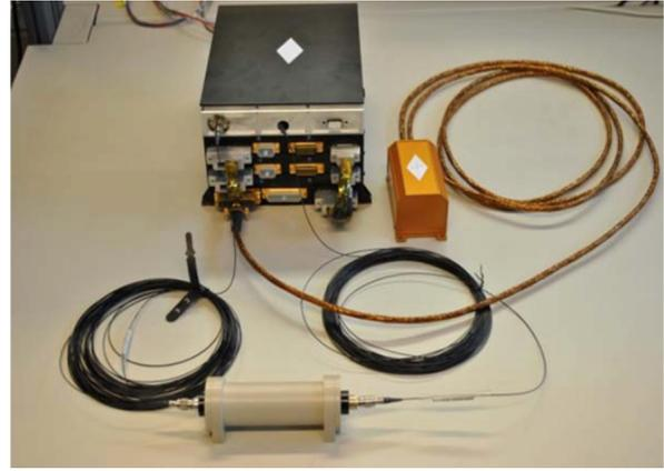
**Fig. 12: Left panel** – Example of the type of solar wind ion detector (flown on Chang'E-1/2) that will be adopted for SMILE LIA. **Right panel** – Example of fluxgate magnetometer (both from CAS/NSSC).
