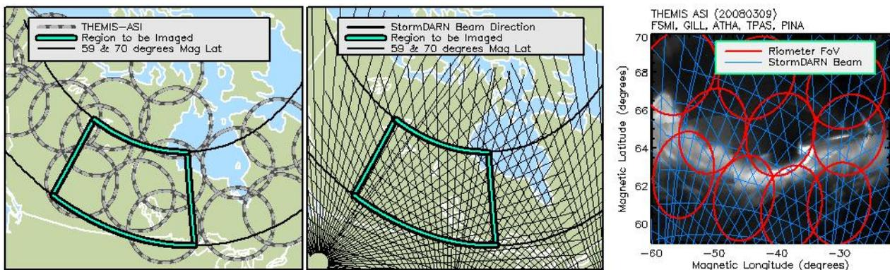
**Figure 6:** TREx imaging region with (left) FoVs of THEMIS ASI and (middle) beam patterns of the NSF funded mid-latitude SuperDARN HF radars. Right) Geomagnetic plot of the target region, SuperDARN beams, and new TREx imaging riometer FoVs, over-plotted on a mosaic of THEMIS-ASI white light images during moderate-high geomagnetic activity.
