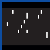
The multi-object slit mask is made, and then inserted at the telescope focal plane
