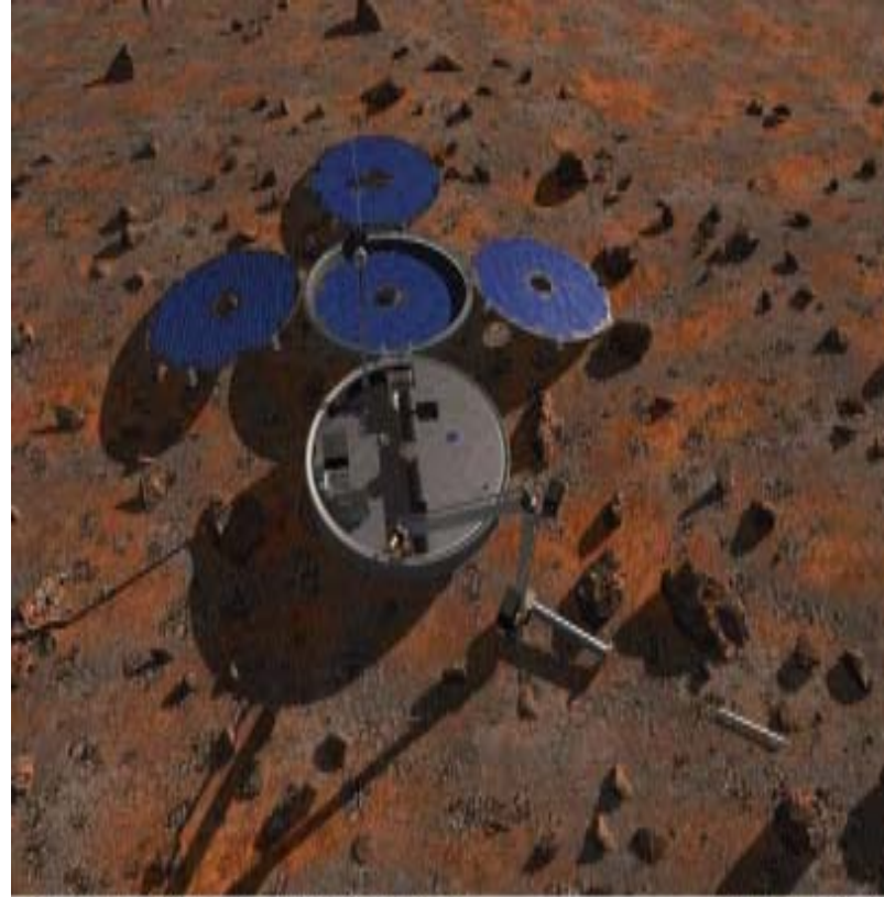
Beagle 2 opens up to expose its solar panels and deploy its instruments
