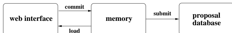
Figure 5: Illustration of the concept of an intermediate memory for proposal information that has not yet been submitted into the proposal database.
