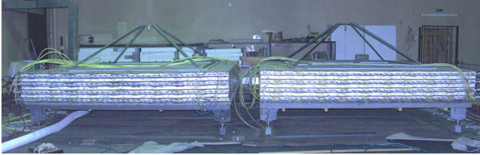
Fig. 3. Two supermodules of muon hodoscope URAGAN [10] which were under operation in December, 2006.
