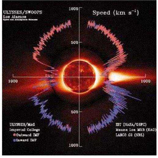
Above plot shows solar wind speed measured during an orbit over the poles of the Sun – solar wind emitted from polar coronal holes is much faster, averaging 800 km s<sup>-1</sup>.
