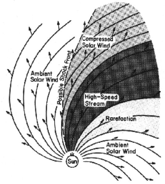
Fast solar wind streams catching up with slower streams cannot mix with the slower stream (frozen-out) Hence the slow stream is compressed and a shock may form (see next section). Slow wind behind the fast wind may cause a rarefaction region of reduced density. These structures may persist for many months and are thus observed every solar rotation (i.e. they corotate with the Sun)
