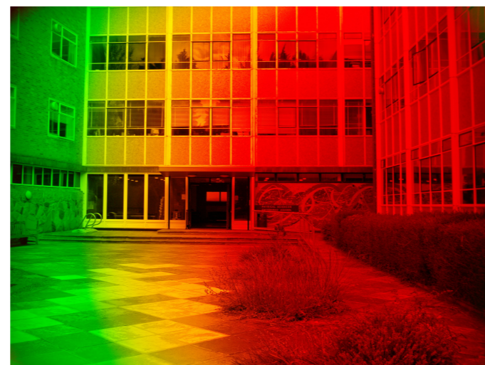
Variable filter in front of a commercial colour camera – showing dispersion across the 2D image.
