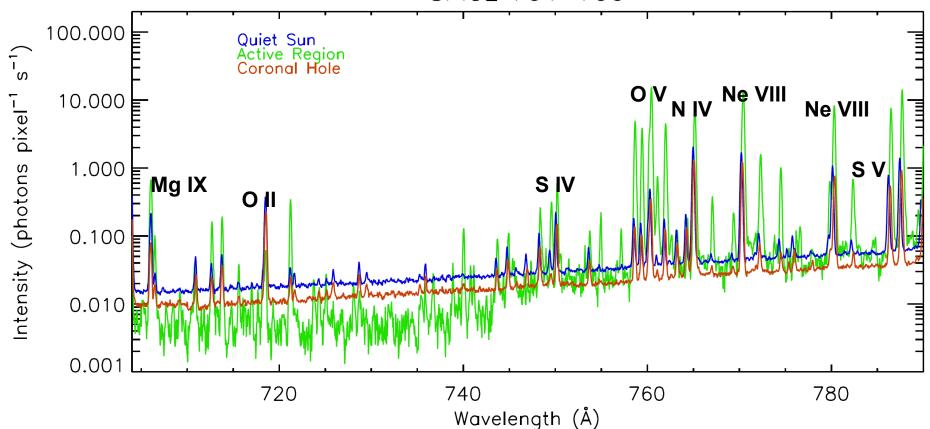
~30 s – 180 s exposure Ne VIII – 600,000 K – outflows in coronal holes Mg IX – 950,000 K – line broadening above the limb Both bands – composition studies
